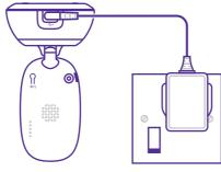
power supply unit item code 089010. mains power socket and switch the socket on. Please use 3 Plug the cable into the Baby unit, then plug it into the
