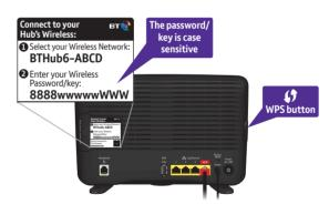
i Prefer a wired connection? Using your Ethernet cable (yellow ends), connect your device to a yellow Ethernet port (1, 2 or 3 only) on the back of your Hub.
