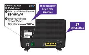
**Prefer a wired connection?** Use your Ethernet cable (yellow ends) to connect your device to any of the vellow Ethernet ports on the back of your Hub.
